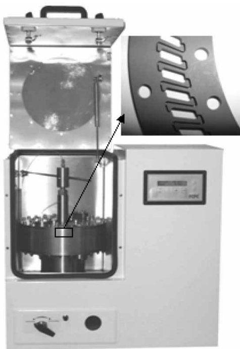
Figure 2. Kromaton Technologies FCPC ® 200 mL rotor and partition disk. Note the connecting ducts centred on the bottom and the top of each cell. The upper and lower cell walls are made of inter-disk Teflon ® gaskets.
